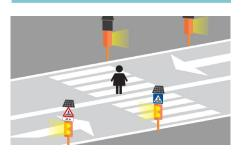
Nr. 02 orange galvanized steel poles (art.21 Highway Code / art.30 implementation regulation) to be positioned near crossings, for each direction of travel. Nr. 02 orange galvanized steel poles (art.21 Highway Code / art.30 implementation regulation) to be positioned about 40 mt. from the crossing, one for each direction of travel.
