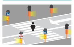
Nr. 04 orange galvanized steel poles (art.21 Highway Code / art.30 Reg. implementation regulation) to be positioned near crossings, two for each direction of travel. Nr. 02 orange galvanized steel poles (art.21 Highway Code / art.30 implementation regulation) to be positioned about 40 mt. from the crossing, one for each direction of travel.
